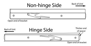
Line up rack slide with slide brackets and push rack in all the way. Pull rack outward all the way to make sure locks are engaged.
