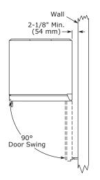
Units have a zero clearance for the door to open 90°, when installed adjacent to cabinets.
