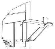
Remove corresponding screws on opposite side of cabinet. On some models there may be a nut behind one or both screws on either side.
