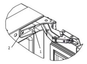
3. Once door is removed, using a Philips Screwdriver remove screws from magnet actuator located on inside and bottom of door. (On Integrated Models magnet actuator will be located on bottom of door.
