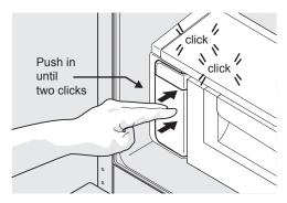
Figure 50 Reinstall water filter
