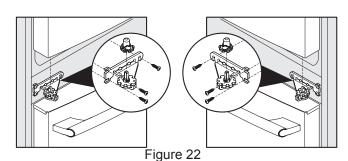
Once both doors are in place, ensure they are aligned with each other and level (please see the "Installation" section for more details), and replace the top hinge cover.
