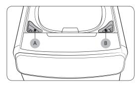
The upper washer provides two cleaning agent compartments: the left-side compartment for bleach, and the right side for fabric softener. You can apply detergent manually into the tub using the provided Aqua Pebble.
