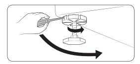
3. When levelling is complete, tighten the nuts using the wrench.
