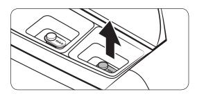
**1.** Open the top-front cover, and then remove the softener cap.
