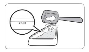
2. Put a recommended amount of liquid or powdered detergent into the provided Agua Pebble. The Agua Pebble has a guide line (marked '20 ml') near its top, which is the max line. Do not exceed the max line.
