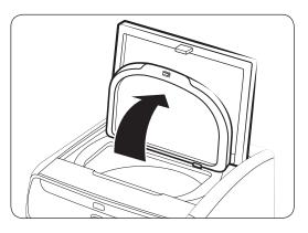
1. Open the top door, and then the protective cover. Remove the Agua Pebble from the fabric softener container.
