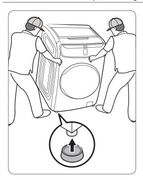
To protect a soft floor or surface, use the provided rubber cups. You don't need to use the rubber cups on a hard floor or on a pedestal.
