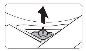
**1.** Open the top door, and then remove the softener cap.
