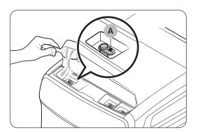
2. Add a recommended amount of liquid or powdered detergent to the detergent compartment. Do not exceed the max line (A).
