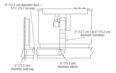
THROUGH FLOOR BETWEEN JOISTS TO OUTSIDE
