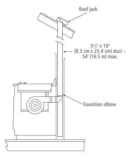
**REAR DUCTING IN WALL TO ROOF**
