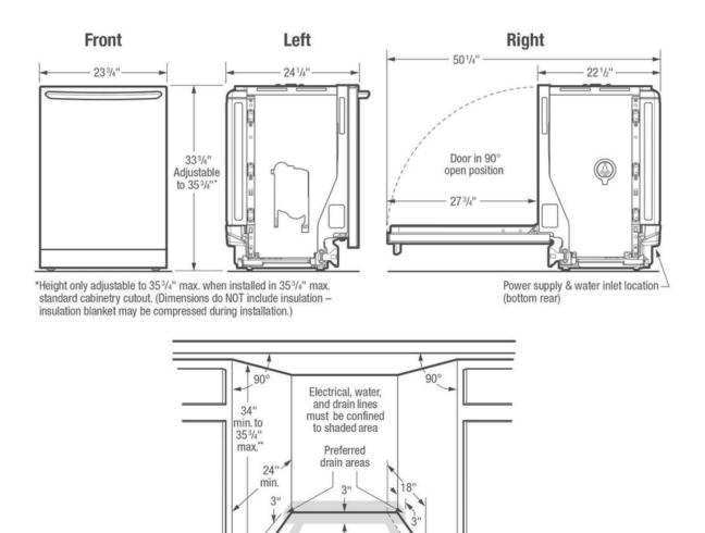
\*\*NOTE: 35<sup>3</sup>/4" max. height for standard cabinetry cutout. (<sup>5</sup>/<sub>16</sub>" min. clearance required from unit to underside of countertop.)
