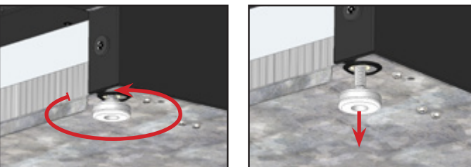
FIG. 2. Turn the leveling legs counterclockwise to raise the unit.
