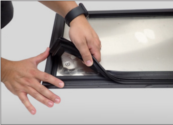
FIG. 3. Pull the gasket from the drawer.
