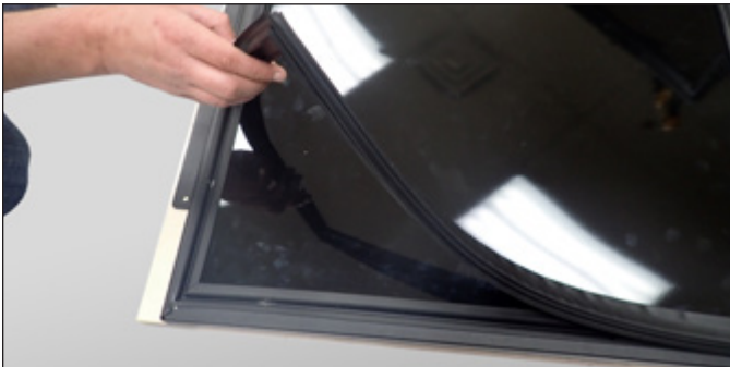
FIG. 3. Pull the gasket from the door.
