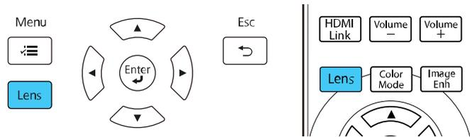
3. Press the **Lens** button repeatedly until **Adjust Zoom** is displayed on the screen.
