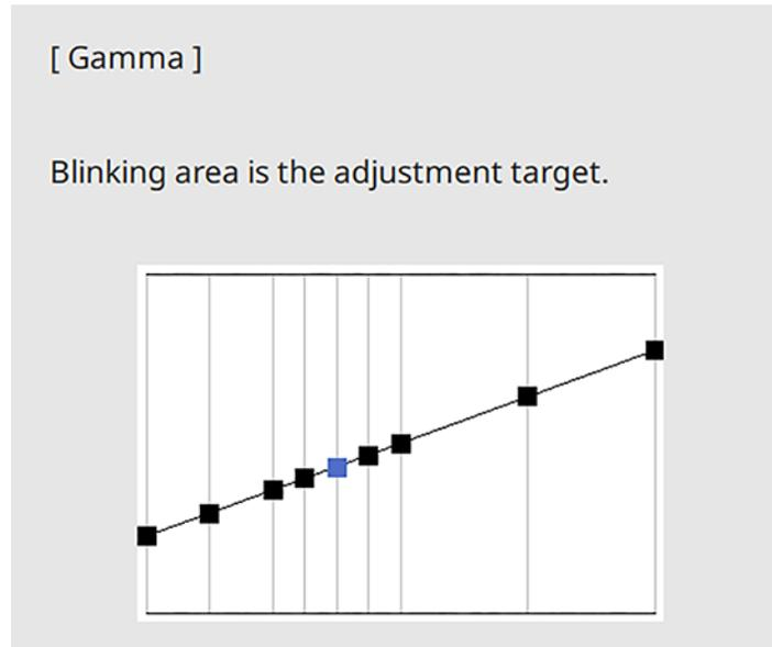
7. Press the left or right arrow button to select the tone you want to change, then press the up or down arrow button to adjust the tone and press **Enter**.
