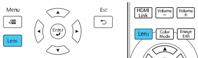
3. Press the **Lens** button repeatedly until **Adjust Focus** is displayed on the screen.
