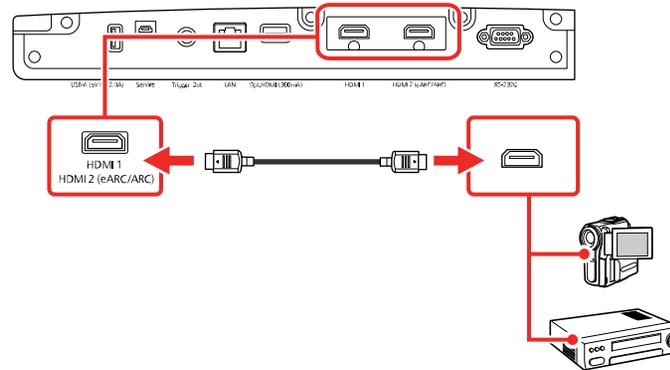
**Note:** When an audio/video source that meets the HDMI CEC standard is connected to the projector's HDMI port, you can use the projector's remote control to control certain features of the linked device by pressing the **HDMI Link** button on the remote control and setting **HDMI Link** to **On**.
