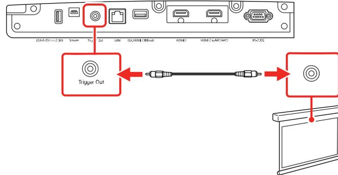
3. Turn on the **Trigger Out** setting in the projector's Operation menu.
