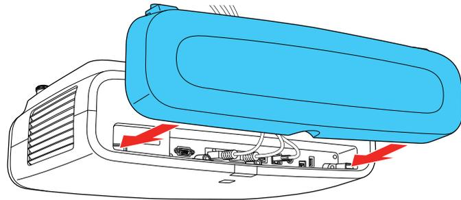
4. Tighten both cable cover screws.
