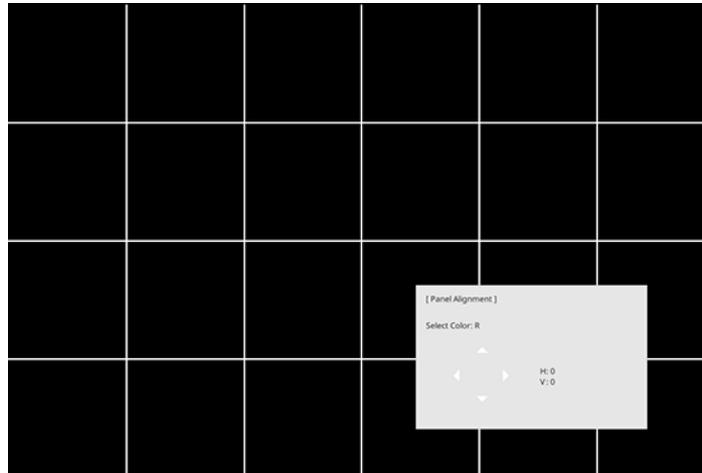
11. Use the arrow buttons on the remote control to adjust the color alignment of the color you selected for the **Select Color** setting.
