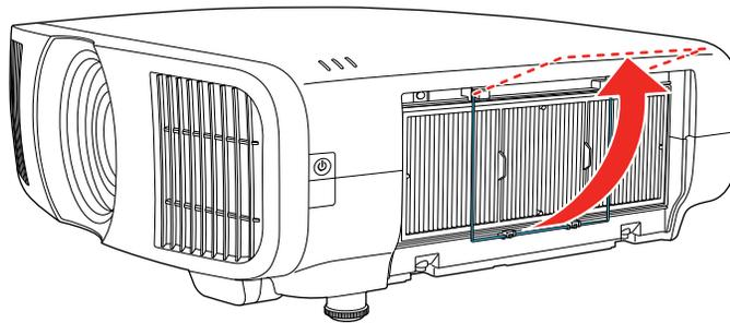
4. Pull the air filter out of the projector.
