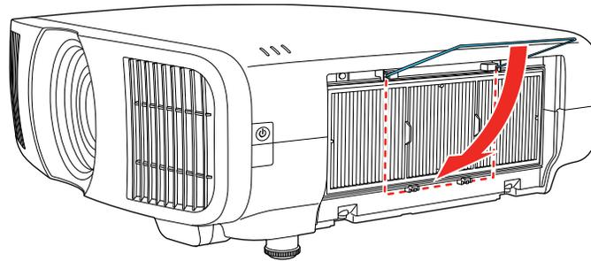
10. Replace the air filter cover and tighten the screws as shown.
