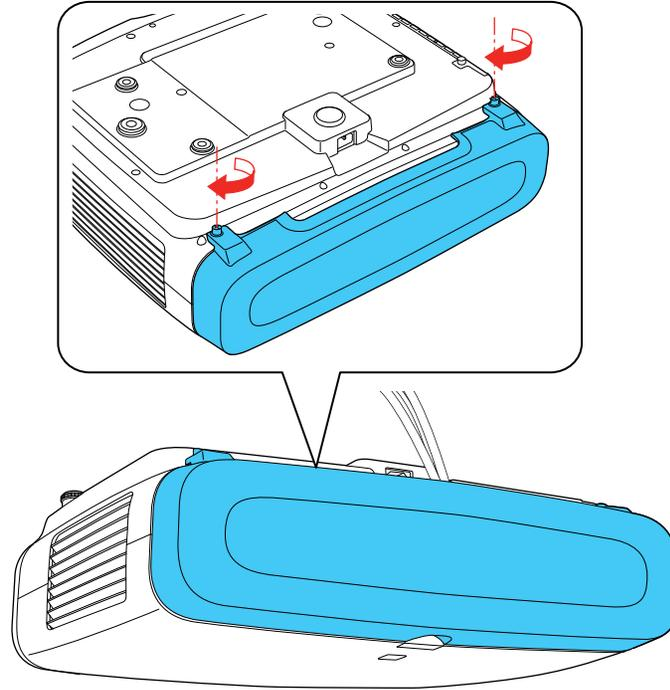
To remove the cover, loosen both screws and pull the cover off of the projector.
