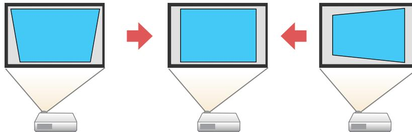
**Note:** Try adjusting the projector's placement and lens shift before using keystone correction. Digital image correction reduces the number of pixels in the image.
