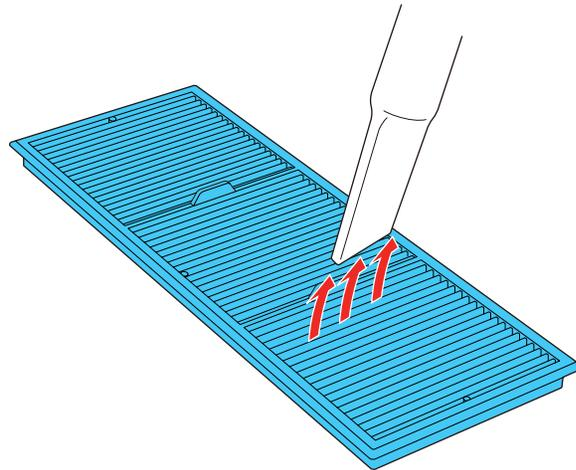
**Note:** If dust is difficult to remove or the air filter is damaged, replace the air filter.
