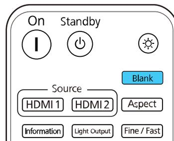
2. To turn the picture back on, press the **Blank** button again.
