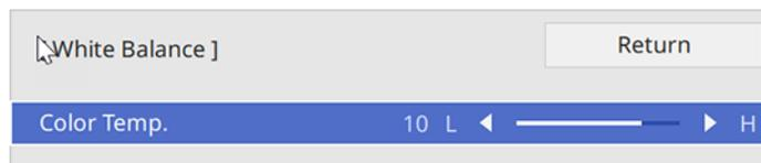
6. Use the left and right arrow buttons to adjust the color temperature. Higher values increase the blue tint, and lower values increase the red tint.
