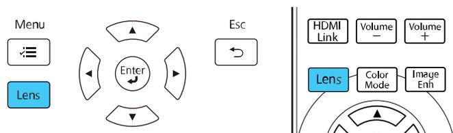
3. Press the **Lens** button repeatedly until **Adjust Lens Shift** appears on the screen.
