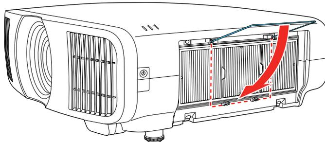
7. Replace the air filter cover and tighten the screws as shown.
