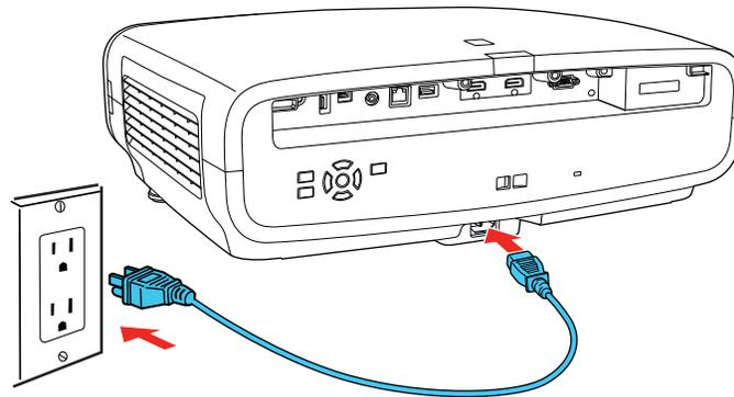
2. Plug the power cord into an electrical outlet.
