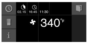
The appliance assumes a waiting mode. The operating mode, the temperature, the cooking time and the end of the cooking time appear in the display. The appliance starts at the calculated time and switches off automatically when the cooking time has elapsed.
