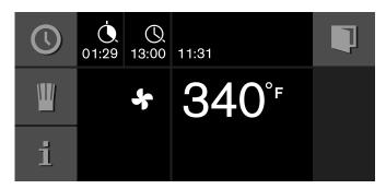
One minute before expiration of the cooking time, the expiring cooking time is enlarged in the display.
