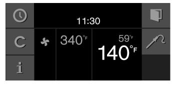
5 The appliance heats with the set heating function. The current core temperature is displayed and, under it, the set core temperature.
