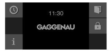
The child lock is activated. The standby screen appears. The 🗗 appears at the top of the display.
