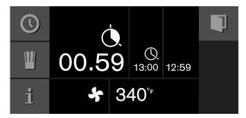
The appliance switches off after expiration of the cooking time. The pulsates and a signal sounds. It goes off prematurely if you touch the  $\checkmark$  symbol, open the appliance door or set the program selection to **0**.
