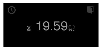
A signal sounds once the time has elapsed. The audible signal ceases if you touch the  $\checkmark$  symbol.
