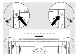
Use the screws supplied to secure the microwave oven to the side walls of the cabinetry through the holes in the oven trim.
