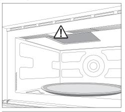
There is a cover protecting the microwave outlet on the ceiling of the oven, which is susceptible to damage.
