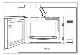
Attach the enclosed quick guide to the frame behind the door (as illustrated), making sure it does not block any of the vents. When installing the microwave oven, ensure that there is unhindered ventilation at the front of the appliance.
