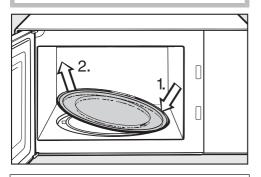
Do not turn the turntable manually, as this could damage the drive motor.
