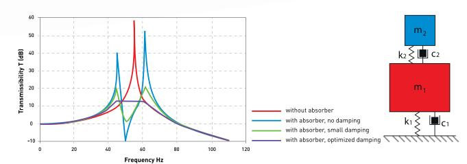
The graph on the left demonstrates the principle of the tuned mass damper. In red, an m1-k1 mass-suspension system displays a pronounced resonance. Adding an m2-k2 device (upper section of the diagram on the right), generates two resonance spikes (represented by the blue curve on the graph). The anti-resonance dip associated with the resonance of the main system produces the green curve. Finally, by tuning the damper, we obtain the purple curve, practically quashing the resonance entirely.
