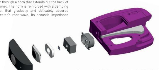
The rear wave from the Beryllium tweeter is gradually absorbed in the first chamber, which in turn transmits to a damped horn that opens onto the rear of the loudspeaker, preventing any feedback from obscuring the incredible definition of the Beryllium tweeter.
